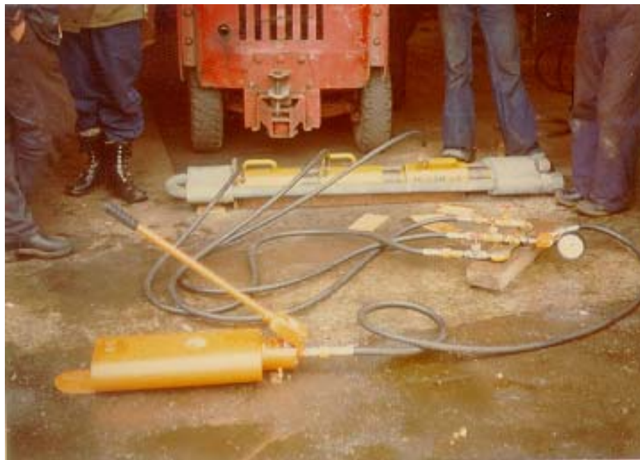
Figure D-2 Testing of hydraulic jacking system by placing jacks in series between two immovable objects.
