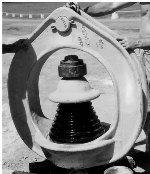
Figure 6-9 Compression cone insulator.
