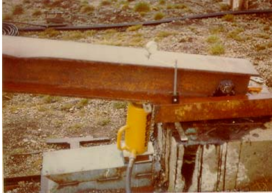
Figure D-3 Testing of rate of descent of a jack by loading it with a metered heavy beam.
